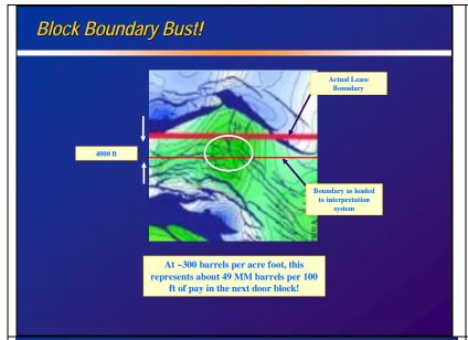
A lease block boundary issue – the Thick boundary line on top is the actual boundary. The thin line below is where the boundary was plotted in the interpretation system. The potential prospect is the oval area, and on the basis of the incorrect lease line location, would not be a suitable target for exploration in our block.
