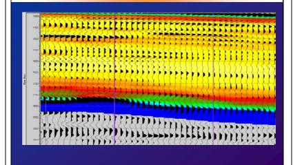
Well data misplaced about 1800 meters – and used for inversion. While one well may not cause too much trouble, 75% of the wells in this field were misplaced. This will create major bias in the inversion and subsequent use of the data for follow on drilling decisions.
