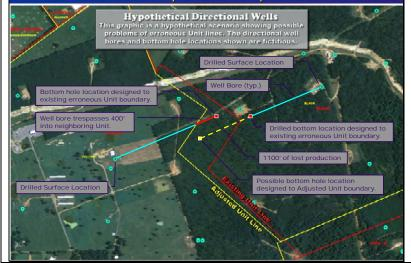
Shows the impact of incorrect well and boundary locations on two hypothetical well plans depending on which way the boundary needs to move to correctly represent the ground truth.
