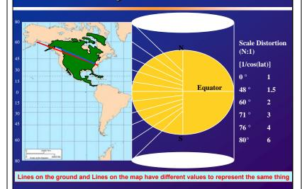
Mercator Projection. Secant of the latitude is used to project onto plane. This causes severe areal distortion in the northern latitudes, but has the property of making lines of constant azimuth straight lines – which is useful for vessel navigation.
