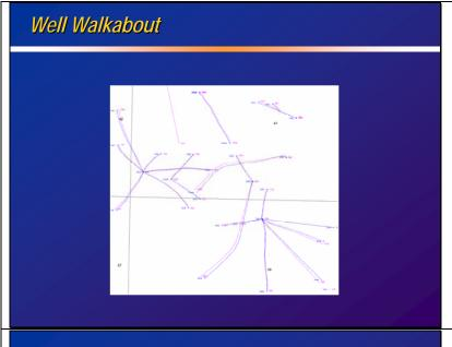
This slide shows 40 well tracks for 20 wells in 2 randomly selected concession blocks in the Gulf of Mexico. These data came from two different commercially available well databases.
