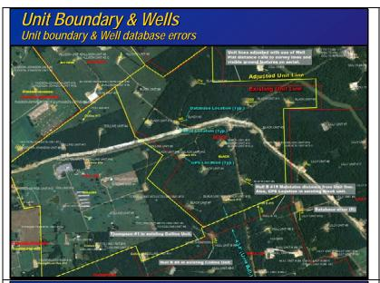
Shows the published grid lines from Tobin (red), versus the adjusted (yellow) based on surveyors well plat distances reversed back from corrected GPS well locations.
