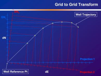
The Blue grid shows the first projection you are using. The red shows the projection you want to change to. The origin is the well reference (KB or Drill Floor or Ground Level). The blue lines show the dEasting and dNorthing for the black dots which define the well trajectory. Grid north is different, since the location of the well in one projection is different relative to the central meridian than the other.
