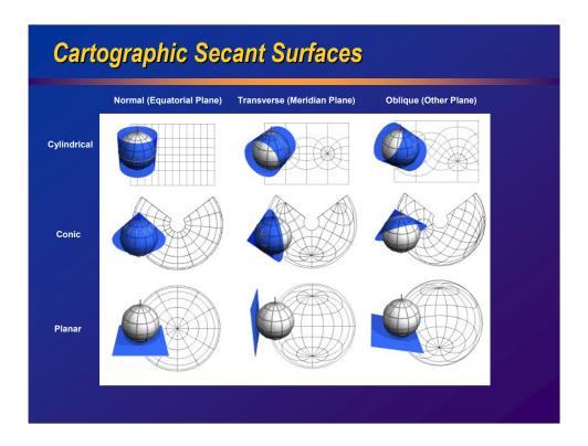
Various methods of projecting data to flat surface. Cylindrical, Conic and planar. Secant vs tangent – secant allows distribution of scale error. Transverse cylindrical touches around a meridian instead of equator. Oblique used for special applications (i.e neither polar or equatorial)
