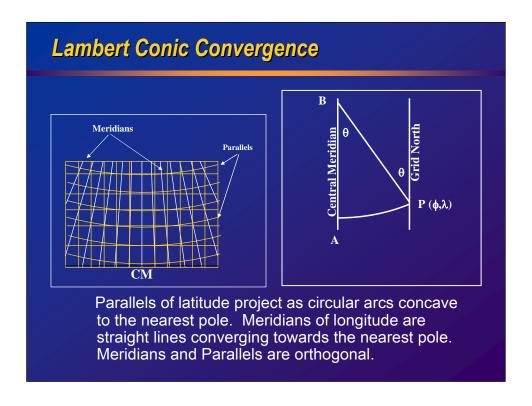
The Lambert projection uses a cone as the projection surface.
