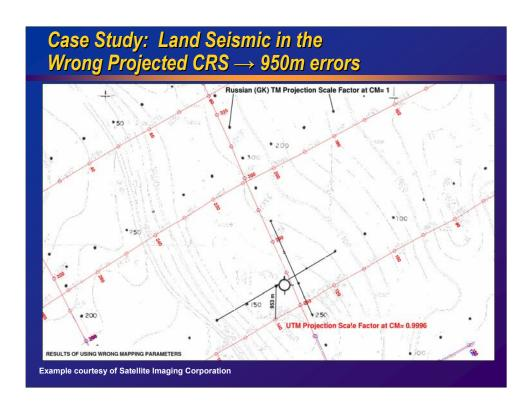
The difference of using two different projections –
