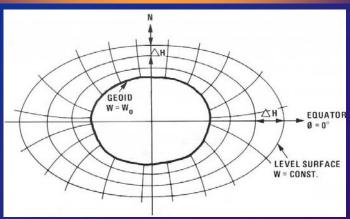
Elevations are measured w.r.t. the geoid, the (physical) surface whose equipotential value (W) is that of Mean Sea Level (W=W<sub>0</sub>). Elevations with respect to the geoid are called "orthometric heights"
