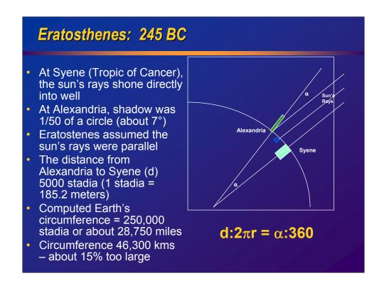
An early "geodesist's" application of scientific principals and simple geometry to obtain an early estimate of the earth's size (assuming that it was a sphere)
