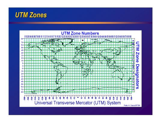
Here is a 'catalogue' diagram of the UTM projection. UTM is a special case of TM, with specifically defined parameters for any region of the world.
