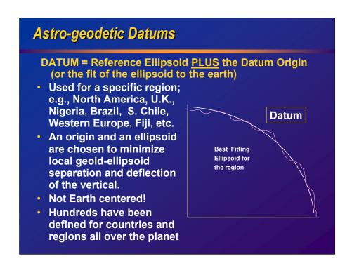
An Astrogeodetic Datum is simply a reference Ellipsoid tied to the earth an a specific point, to best fit mapping that specific area.
