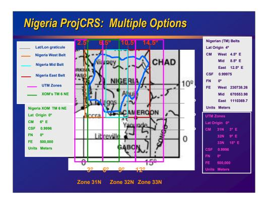
Here is how the Nigeria projected CRS fit together.
