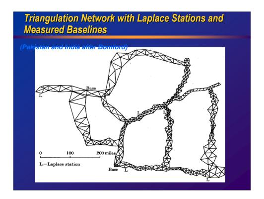
This represents a section of the Geodetic Traverse used to provide base surveys of India and Pakistan.
