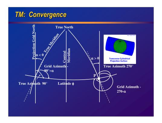
Transverse Mercator projection is derived using the cylindrical method rotated so that the point of tangency or secancy is around a meridian through the poles instead of the equator (see inset)
