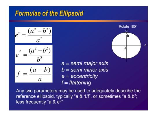
Different software packages require different ellipsoid entry parameters. Some require "a" and "1/f". Others want "a" and "b". Yet others ask for "a" and "e".
