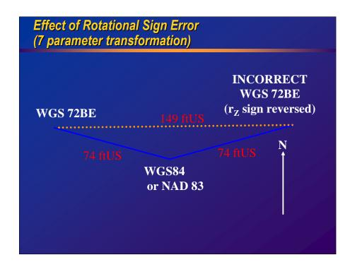
Using the incorrect 7-parameter transformation method (Position Vector 7 parameter transformation vs. Coordinate Frame Rotation) will cause the rotational parameters to be reversed, thus causing twice the error of just leaving out the term.
