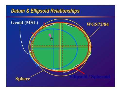
The best-fit sphere "misses" the poles by about 10 km (6 miles); the actual polar radius is much shorter than the equatorial radius.
