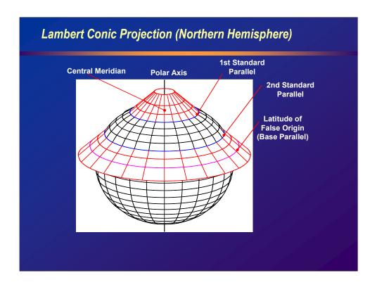
Fitting a cone to a reference ellipsoid (representing the earth's geoid) yields a Lambert Conic Conformal Projection. If the cone is tangential to the ellipsoid surface this becomes a Lambert (Single Standard Parallel) projection. More commonly, the cone will cut into the ellipsoid, yielding a Lambert Two Standard Parallel Projection.
