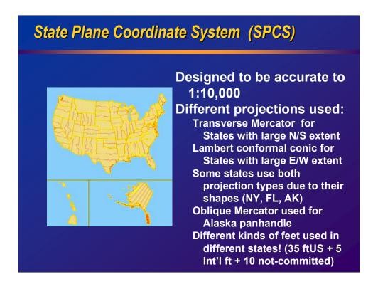
The United States State Plane Coordinate System used both Lambert and TM projections.
