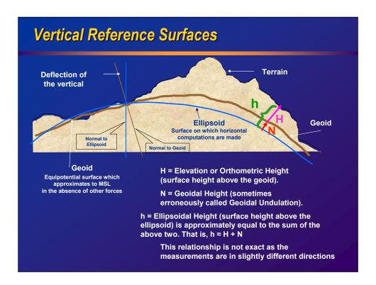
You have seen a similar slide earlier, showing the fundamental issues of establishing a local Geodetic Datum. The slide is shown again here but modified to illustrate the vertical reference surfaces and the relationships between them.
