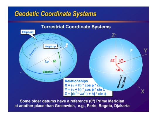
Here are two main coordinate systems used to represent three-dimensional positions on the earth – shown diagrammatically
