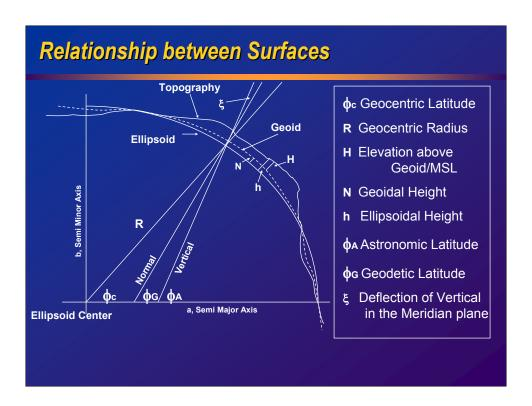
The geocentric latitude is simply a line to the center of the ellipsoid from the point.
