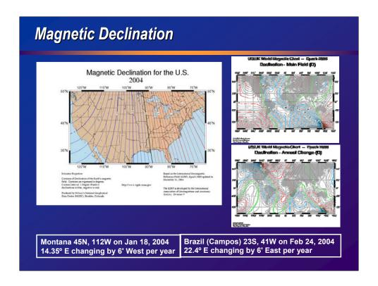
These diagrams show the magnetic declination in USA and the world. The third diagram shows the world rate of change of magnetic declination on an annual basis.
