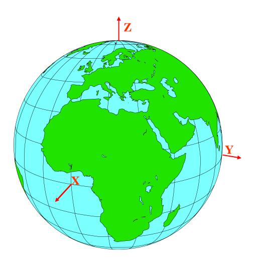
The Z-axis extends from the geocenter north along the spin axis to the North Pole. The X-axis extends from the geocenter to the intersection of the Equator and the Greenwich Meridian. The Y-axis extends from the geocenter to the intersection of the Equator and the 90E meridian.
