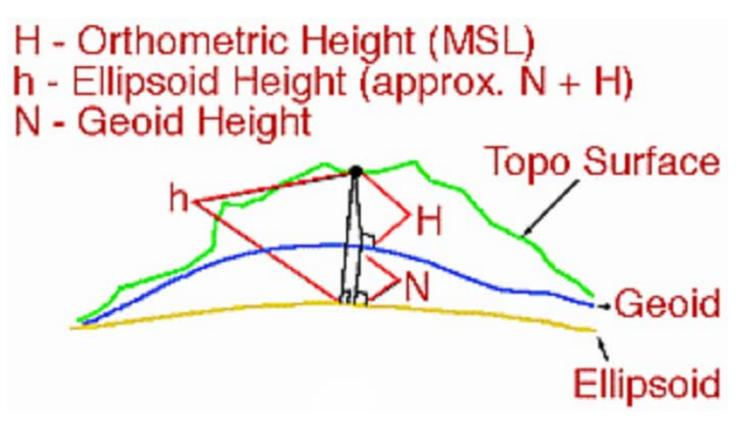
A more closer look at relationships among elevation (orthometric height), ellipsoidal height and geoidal height (undulation). Geoidal heights are determined with a geoidal model such as EGM96.
