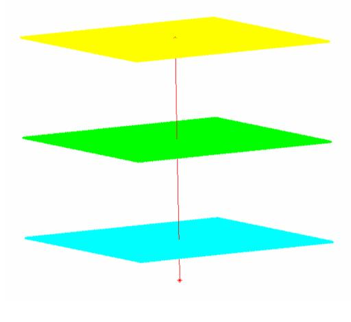
This cartoon of the reservoir off Ujung Pandang is in a G&G's typical VE perspective. It is 10km by 10km horizontally in plan view with three interpreted horizons: a yellow sealevel surface, basement 10km deep in blue and one in between in green. A well is drilled through basement.
