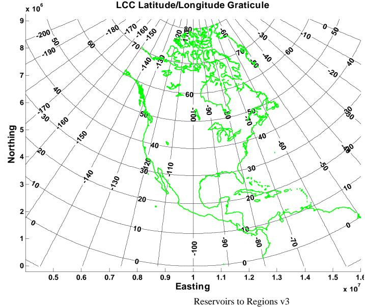
Meridians are straight lines and parallels are curved. They intersect orthogonally. **Distortion** is managed by selection of grid parameters
