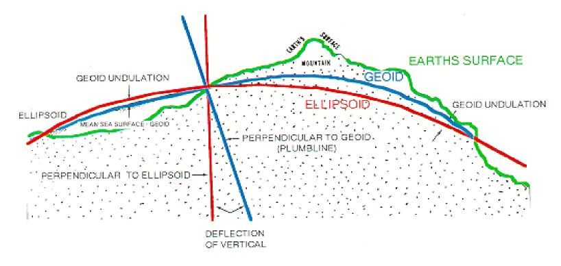
Geoidal undulation (or geoidal height) is the difference between the surface of geoid and the surface of the ellipsoid. EGM96 is the best public-domain model of world-wide geoidal heights. Some local datums have poor information about geoidal height.
