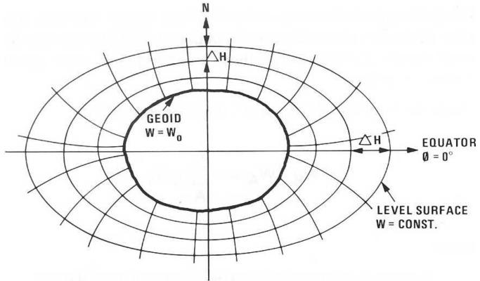
Elevation is measured along the (slightly curved) vertical, which is perpendicular to the irregularly layered geopotential surfaces of the earth. The geopotential surface at mean sea level is called the geoid. (Graphic from Hoar, 1982.)
