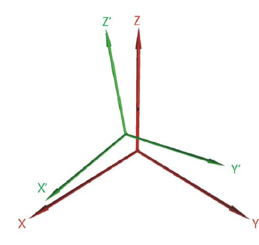
The relationship between two geodetic datums can be described by the 7 parameters required to transform their Geocentric CRSs into alignment (3 translations, 3 rotations and 1 scale change). For example, the red Geocentric CRS might be WGS84 and the green might be ED50.
