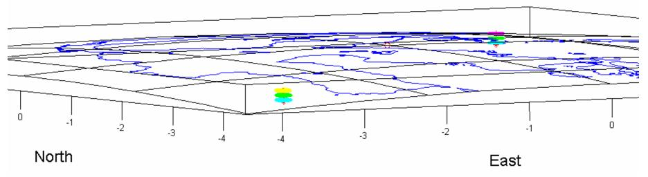
The curvature of the earth is preserved without any mapping distortion in this regional perspective that captures both reservoirs and - in principle - all the modeled geology in between. The G&G can zoom into any area of interest, in as much detail as desired, and perform any volume computation in true meters. Or the G&G can zoom out in order to evaluate regional trends.
