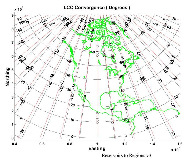
The red lines contour azimuth difference between grid and true north (i.e., convergence of the meridians) in degrees, varying (W to E) from -70° => 0° =>  $+70^{\circ}$
