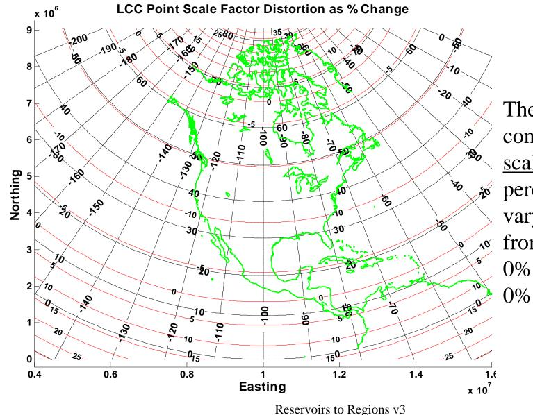
The red lines contour <u>linear</u> <u>scale change</u> as a percentage, varying (N to S) from +35% =>0% => -10% =>0% => +15%.
