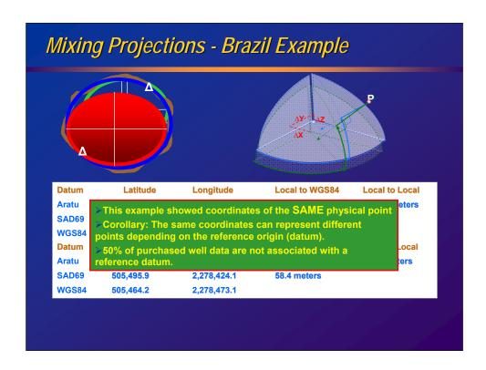
This shows the same example as we saw in the geodesy module, but includes now, the projection coordinate differences.
