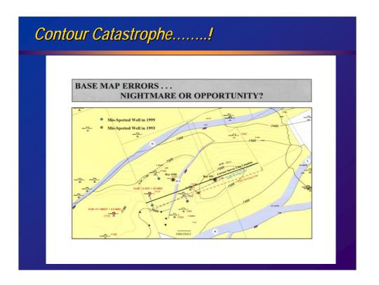
4 wells repositioned  $\sim$ 500 ft, due to grid error discovered by geologist's field visit, allowed for re- contouring and subsequently discovery of 2 major gas fields.
