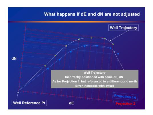
Here is what happens if you use the blue dEasting and dNothing on the red projection. It rotates the well trajectory in space. Remember that the well trajectory doesn't move, we are changing the north reference, when we change the projection. As you can see the potential damage to the integrity of the well trajectory position could be severe (increase with offset from the well reference point.
