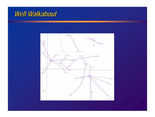
This slide shows 40 well tracks for 20 wells in 2 randomly selected concession blocks in the Gulf of Mexico. These data came from two different commercially available well databases.
