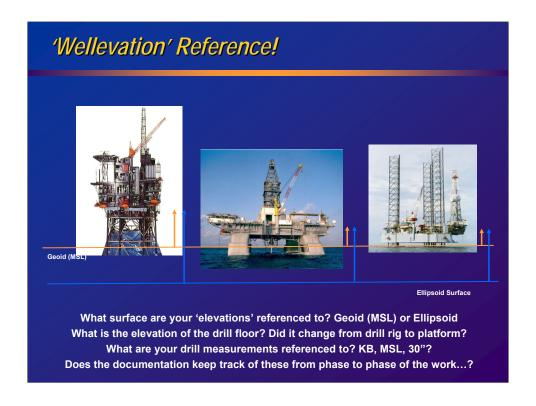
Managing the vertical referencing can be a challenge as a project proceeds. Referencing everything to the KB or MSL in the drilling stage and not keeping track can lead to mis-referencing of elevation at a later stage when a platform is installed.
