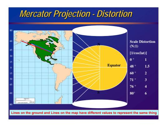
Mercator Projection. Secant of the latitude is used to project onto plane. This causes severe areal distortion in the northern latitudes, but has the property of making lines of constant azimuth straight lines – which is useful for vessel navigation.
