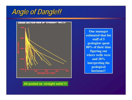
The above diagram shows the result of re-surveying all the 'straight' (un-deviated) wells on a prospect!
