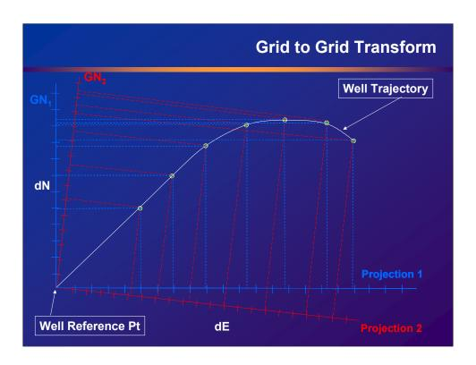
The Blue grid shows the first projection you are using. The red shows the projection you want to change to. The origin is the well reference (KB or Drill Floor or Ground Level). The blue lines show the dEasting and dNorthing for the black dots which define the well trajectory. Grid north is different, since the location of the well in one projection is different relative to the central meridian than the other.
