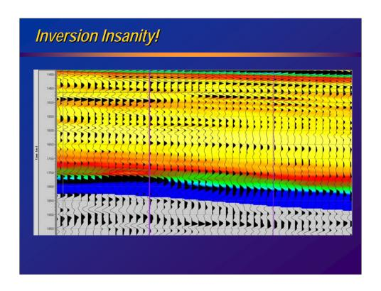
Well data misplaced about 1800 meters – and used for inversion. While one well may not cause too much trouble, 75% of the wells in this field were misplaced. This will create major bias in the inversion and subsequent use of the data for follow on drilling decisions.
