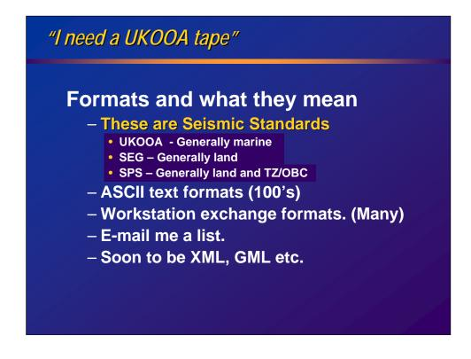
Positioning data is exchanged in multiple formats. There are standard exchange formats designed for seismic positioning data. The common names are UKOOS, SEG and SPS.
