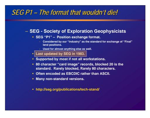
This is far and away the number one format in use. It is used for land, marine, transition zone and ocean bottom seismic data.
