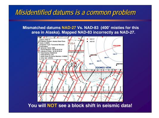
This is an example of incorrectly mapping lat, lon coordinates. The project has been defined as Alaska State Plane Zone 4, which is a Transverse Mercator projection. For this project that projection is referenced to the North American Datum of 1927, which is further referenced to the Clark 1866 Ellipsoid.
