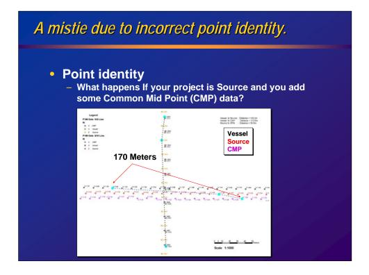
This is an example of three sets of coordinate information from a typical 3D marine survey.
