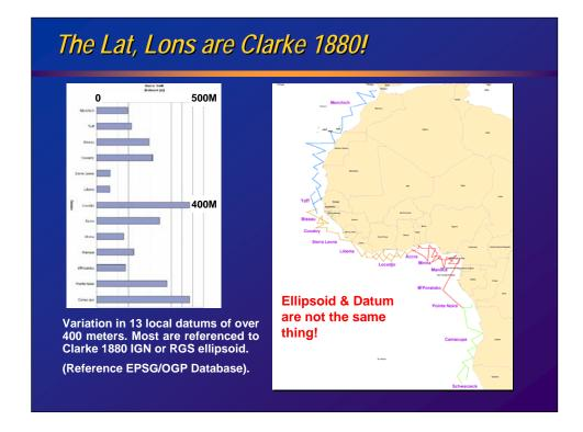
In this slide we see what misidentifying datums in West Africa can potentially cause. Here are 13 commonly used datums, most of which are referenced to a similar or only slightly different ellipsoid. The reality is many datums share common ellipsoids and can have quite different geodetic coordinates. Converting an X,Y to a Latitude Longitude correctly and not knowing the datum might lead to an error in positioning.
