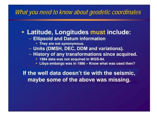
These are the basic requirements to identify which datum and ellipsoid a set of latitude and longitude coordinates belong to. Without this identity information, the potential for misuse, misidentification and error is maximized.
